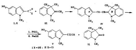
Compounds V and VI were separated by column chromatography. The yield of ethynylindole V was 80%, based on the aminoketone IV, or 55% based on the starting acid I. Its structure was confirmed by elemental analysis and spectral data, the results of which are given in the experimental part.
